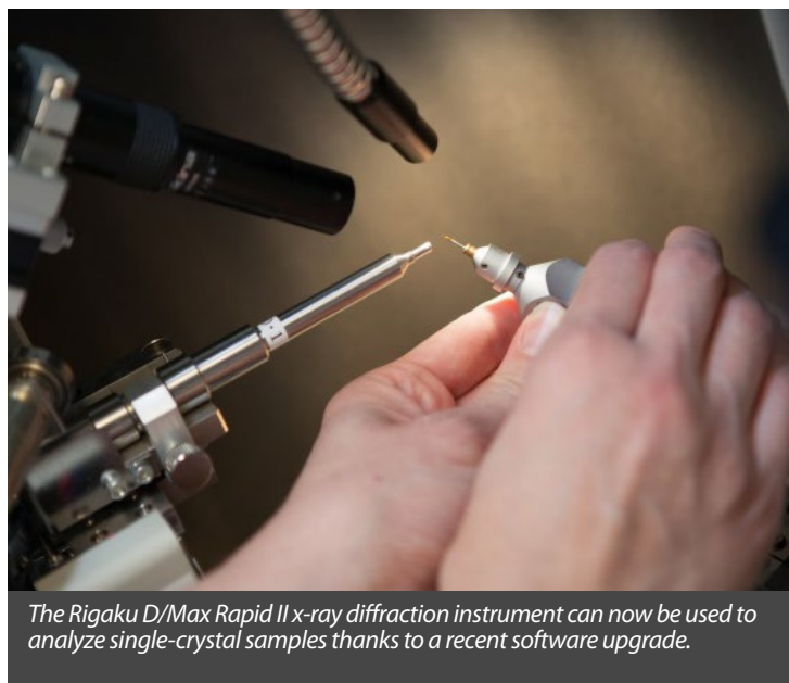
X-rays are diffracted from a single crystal, and the spots they create on the imaging plate are used to determine the atomic structure of the crystalline material.
